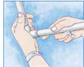
*PVC: 2. Slip pipe into fitting and wipe off excess solvent.*
