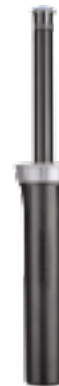
PROS-06-PRS40-CV Retracted height: 8¾" Pop-up height: 6" Exposed diameter: 2¼" Inlet size: ½"
